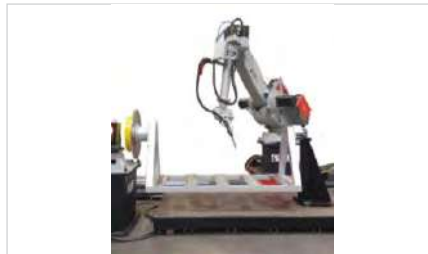
Manufacturing cell additive metal parts > 5 m (Polyshape)
