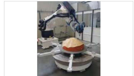
Multifunctional machining cell for composite (Nimitech, Lauak)
