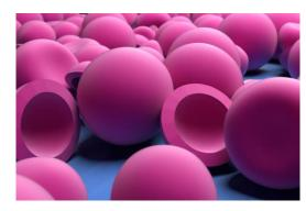
Thermochromic microcapsules absorbing and reflecting light
